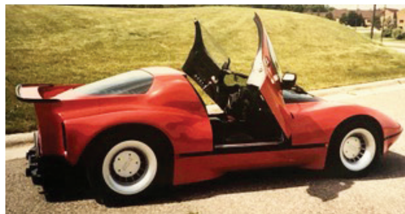
Two gas struts per door, single hinge. (Building doors aren't fun!)
