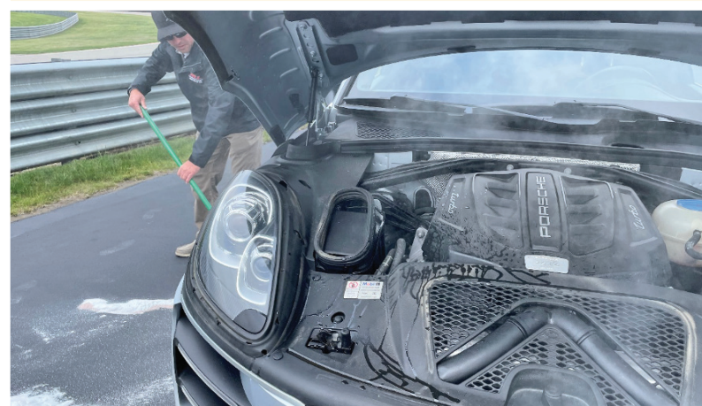
In May 2023, at M1 Concourse, a small plastic coolant pipe had blown and sprayed coolant around the engine, turbos, and transmission.
